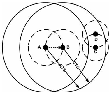
Figure 1 - The IEEE 802.11 approach. Solid lines represent the receiving areas of the RTS and CTS frames when the maximum transmission power is used, while dashed lines represent the transmission ranges of the nodes when the minimum required power for coherent reception is used.
