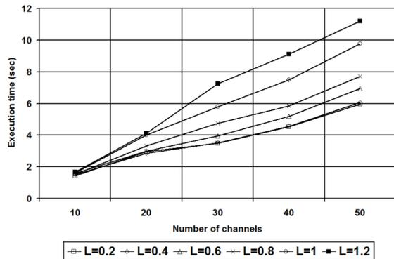
Fig. 5: The average execution time per connection request versus the number of available channels  $W$  per fiber.
