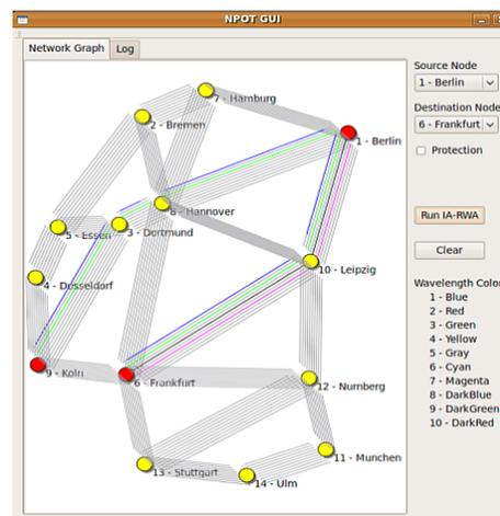
Fig. 3: The established lightpaths on IALCE's GUI.
