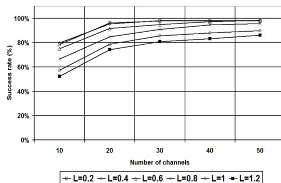
Fig. 4: The success rate versus the number of available channels  $W$  per fiber.
