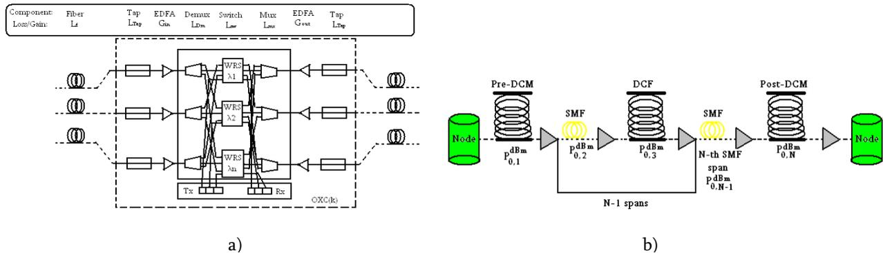
Figure 1: a) Components and their loss/gain parameters in a OXC [7], b) Link model
