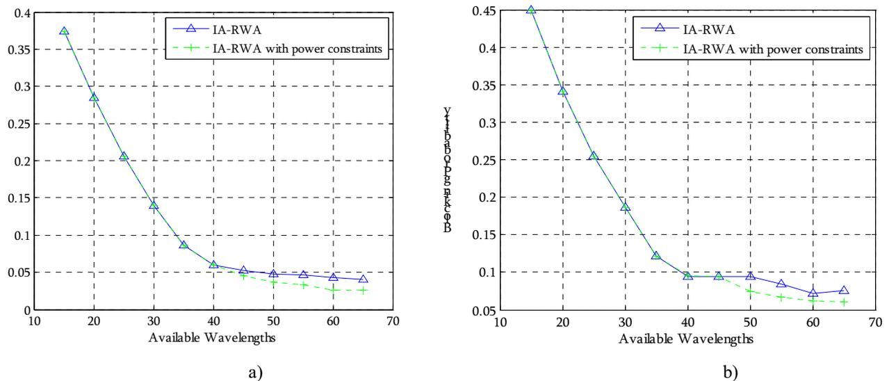
Figure 4: Blocking probability with the available wavelengths in the network, (a) with reroutings, (b) no reroutings (load=400).
