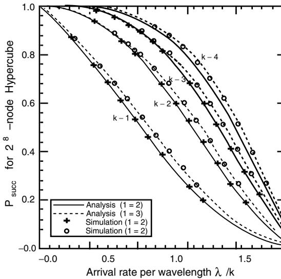
Figure 12.9 Analytical and simulation results for  $P_{succ}$  vs. the arrival rate per wavelength  $\lambda/k$ , for a  $2^8$ -node hypercube network, using adaptive VCD routing.
