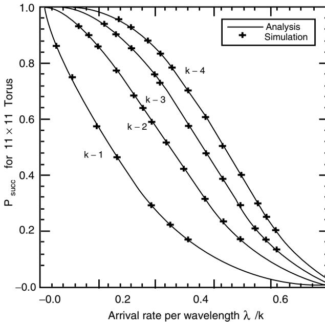
Figure 12.7 Analytical and simulation results for  $P_{succ}$  vs. the arrival rate per wavelength  $\lambda/k$ , for an  $11 \times 11$  torus network, using oblivious (X-Y) routing.
