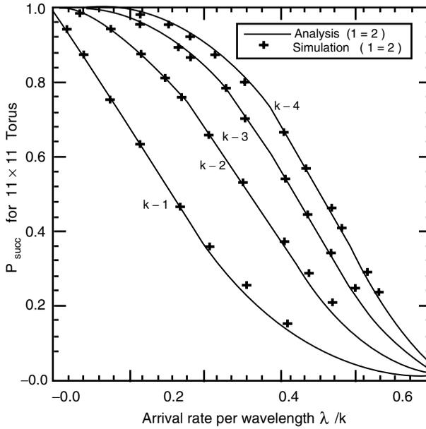
Figure 12.8 Analytical and simulation results for  $P_{succ}$  vs. the arrival rate per wavelength  $\lambda/k$ , for an  $11 \times 11$  torus hypercube network, using adaptive VCD routing.
