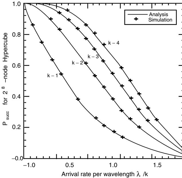
Figure 12.6 Analytical and simulation results for  $P_{succ}$  vs. the arrival rate per wavelength  $\lambda/k$ , for a  $2^8$ -node hypercube network, using oblivious routing.
