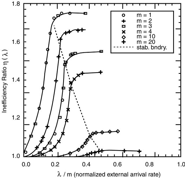
**Figure 12.5** Performance results for the VCD protocol, illustrating the inefficiency ratio  $\eta(\lambda)$  as a function of the normalized arrival rate per unit of link capacity  $\lambda/m$ , for an  $8 \times 8$  MS network and several values of  $m$ . The dashed lines correspond to the stability boundary.
