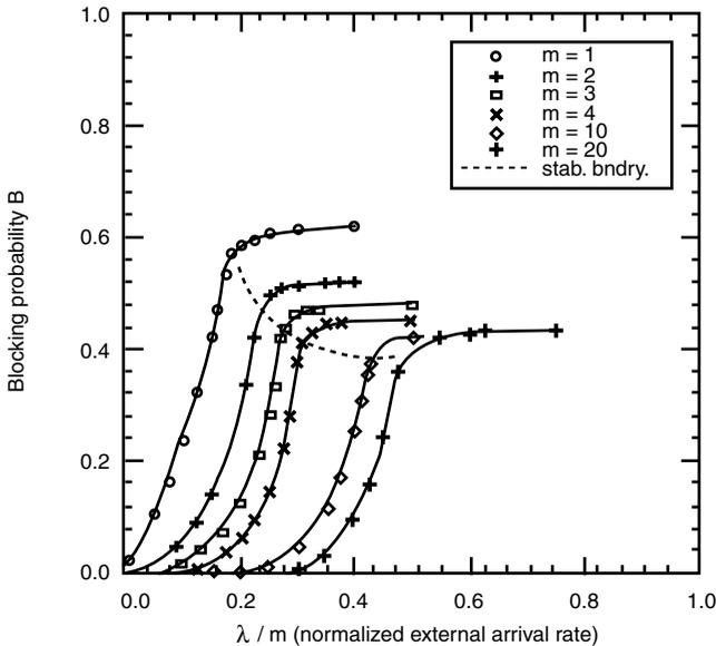
Figure 12.4 Performance results for the VCD protocol, illustrating the blocking probability  $B$  as a function of the normalized arrival rate per unit of link capacity  $\lambda/m$  for an  $8 \times 8$  MS network and several values of  $m$ . The dashed lines correspond to the stability boundary.
