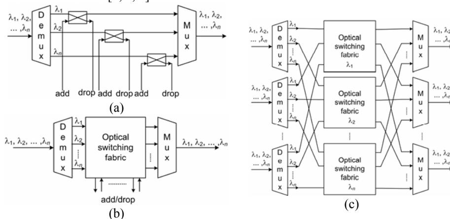
**Fig. 5.1.** (a) OADM with switching elements (b) OADM with the switching fabric (c) OXC with separate switching fabrics for each wavelength.
