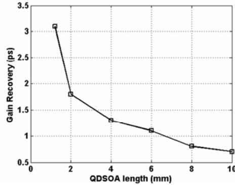
Fig. 5.4. QDSOA gain recovery time as a function of the device length.
