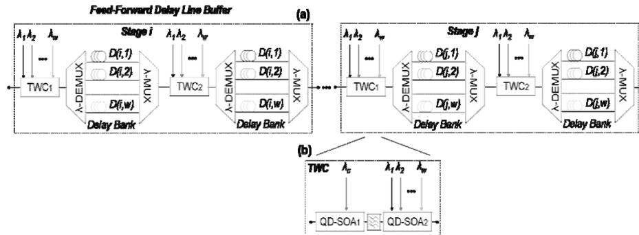
**Fig. 5.2.** (a) The structure of each delay stage. (b) The QDSOA tunable wavelength converter (TWC) setup.  $\lambda$ -MUX/DEMUX are the wavelength multiplexers and demultiplexers, respectively [17].
