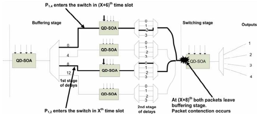
**Fig. 5.8.** The packet contention in the switch with parallel optical buffers. Both packets leave buffering stage at the same time slot and the packet contention appears on the input of the third QD-SOA.
