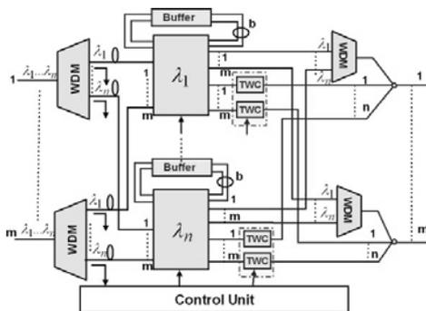
**Fig. 5.16.** OPS architecture A1 based on optical buffers and tunable wavelength converters
