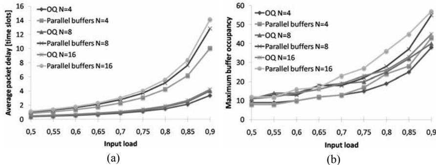
**Fig. 5.9.** Comparison of (a) average packet delay and (b) maximum buffer occupancy for  $b = \infty$ , versus input load for different switch sizes.
