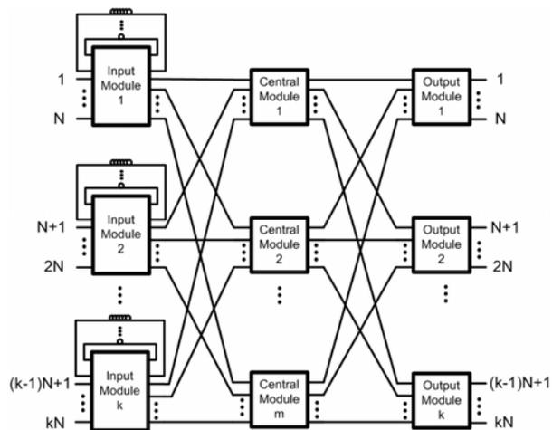
Fig. 5.11. Three-stage shared-FDL-IM optical Clos-Network
