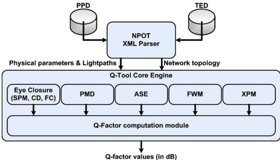
Fig. 3 Building blocks of NPOT Q-Tool module (Q-Tool core engine)
