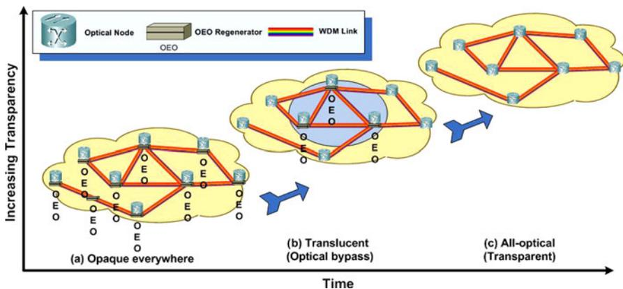
**Fig. 1** Evolution of optical networks from (a) opaque, to (b) translucent (optical bypass), to (c) all-optical (transparent)
