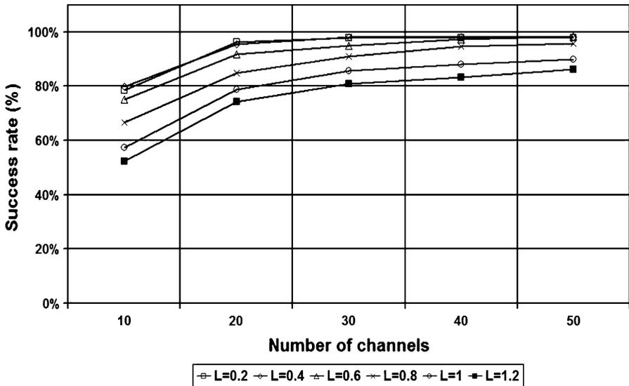
Fig. 9 The success rate versus the number of available channels  $W$  per fiber
