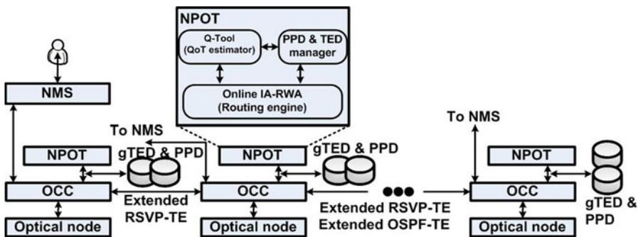
Fig. 5 Distributed control plane integration scheme
