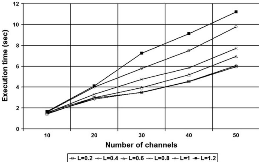
**Fig. 10** The average execution time per connection request versus the number of available channels  $W$  per fiber
