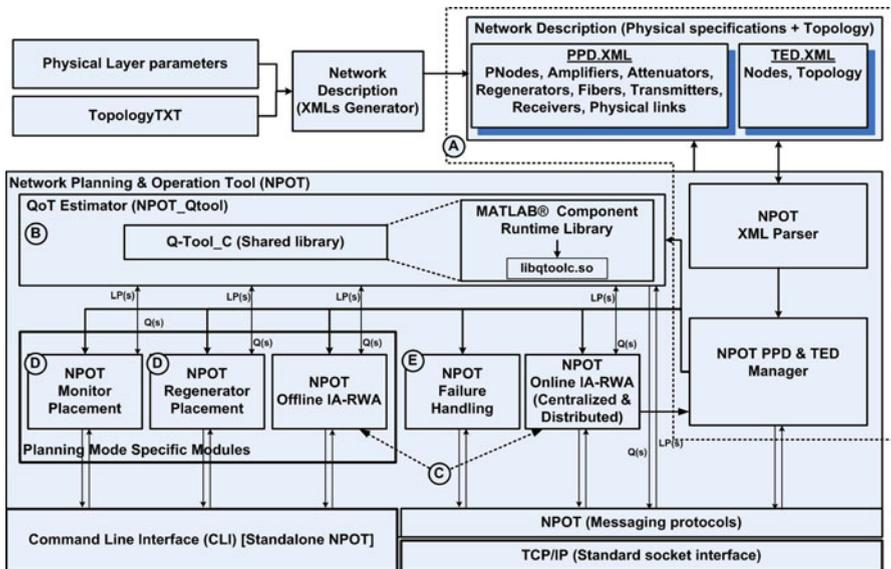
**Fig. 2** Anatomy of DICONET Network Planning and Operation Tool (NPOT): (A) network description repositories, (B) QoT estimator, (C) IA-RWA engines, (D) component placement modules, and (E) failure handling module
