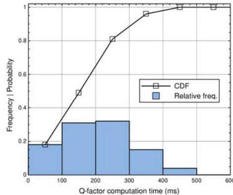
Fig. 5. Relative frequency and CDF of the Q-factor computation time with FPGA-acceleration (load=70 Erlang).
