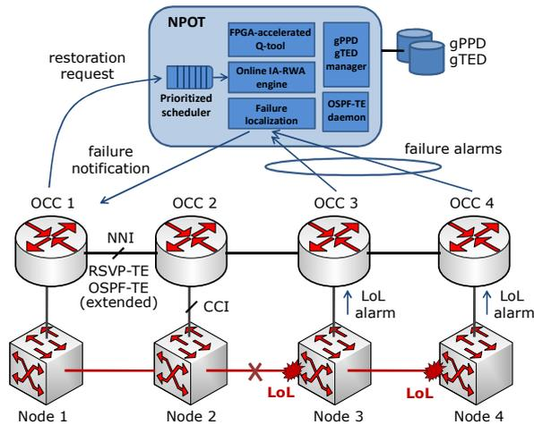
Fig. 1. Centralized restoration example: a bidirectional lightpath is established from node 2 to 4 and a failure occurs between nodes 2 and 3.
