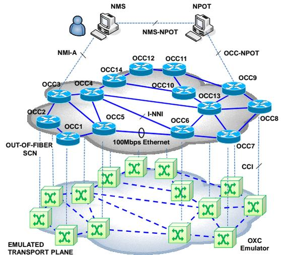
Fig. 2. The DICONET test-bed used for the experiments: A 14-node meshed transport plane with 23 links is emulated.
