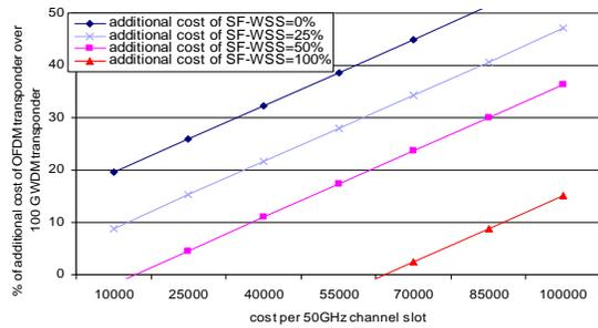
Fig 3. Percentage of additional cost of the SF transponder over the cost of the 100 Gbps transponder as a function of the cost of the 50 GHz slot, for different SF-WSS extra cost percentages and for load=5.
