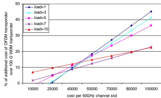
Fig 2. Percentage of additional cost of the SF transponder over the cost of the 100 Gbps transponder as a function of the cost of the 50 GHz slot, for different traffic loads and 50% SF-WSS extra cost.
