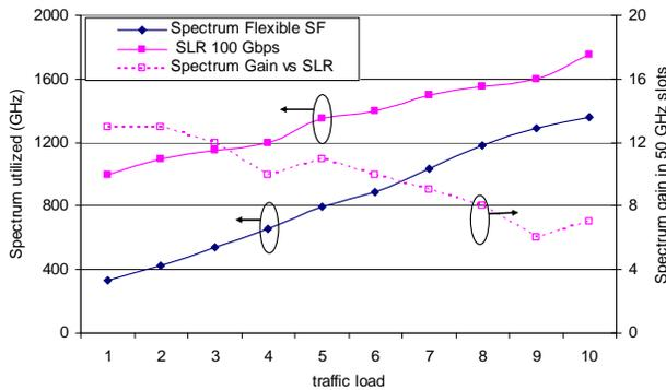
Fig 1. Spectrum utilization and spectrum gain (in 50GHz slots ) of the SF network as opposed to a SLR 100 Gbps system for different traffic loads.
