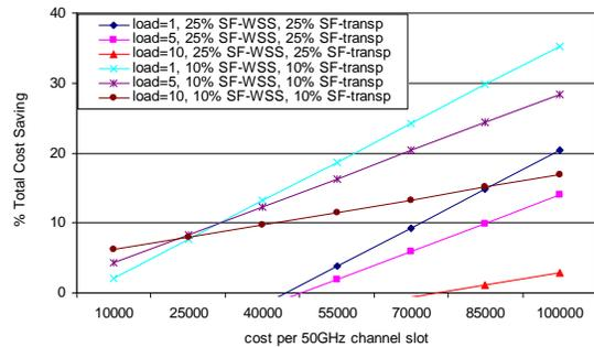
Fig 4. Percentage of total network cost saving as a function of the cost of the 50 GHz slot, for different SF-WSS and different SF-transponder values.
