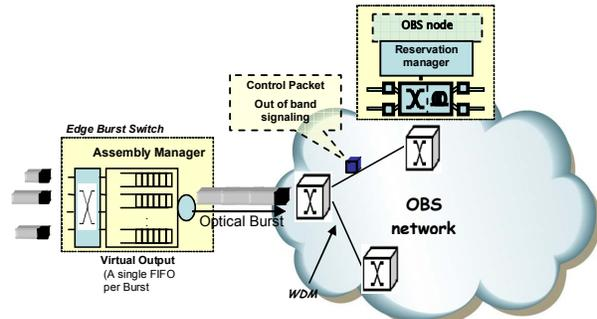
Figure 1: The architecture of a typical OBS network.
