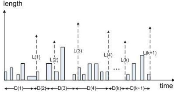
Figure 2: Prediction is performed based on the  $k$  previous burst lengths and assembly durations.
