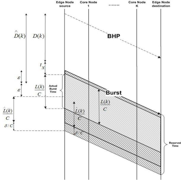
Figure 3: A successful reservation for the  $T_{AVE}$  burst assembly algorithm, using two predictive filters. One filter predicts the burst length  $\hat{L}(k)$  and the other the burst assembly duration  $\hat{D}(k)$ .
