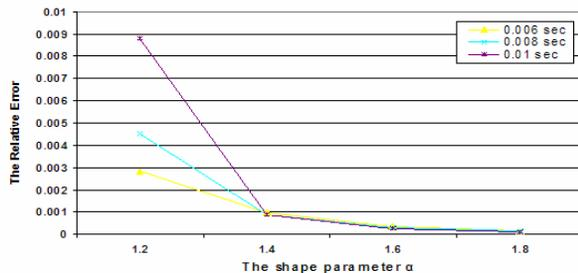
Figure 4: The relative error of the burst length prediction versus the shape parameter  $\alpha$ , for three different values of the burst assembly duration  $D = T_{MAX}$  for the T<sub>MAX</sub> assembly algorithm.
