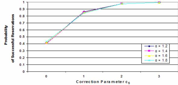
Figure 5: The probability of successful reservations versus the correction parameter  $c_\delta$ , for different values of the shape parameter  $\alpha$  for the T<sub>MAX</sub> assembly algorithm. The burst assembly period was  $D = T_{MAX} = 0.006$  secs.
