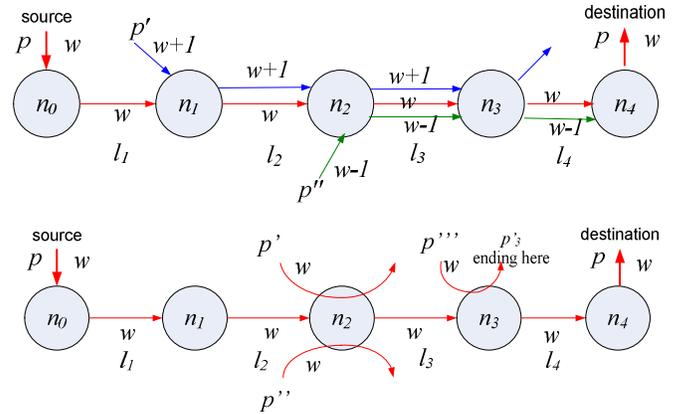
Fig 2: (a) Adjacent channel interference on lightpath  $(p,w)$  by other lightpaths, and (b) Intra-channel XT interference on lightpath  $(p,w)$  by other lightpaths.
