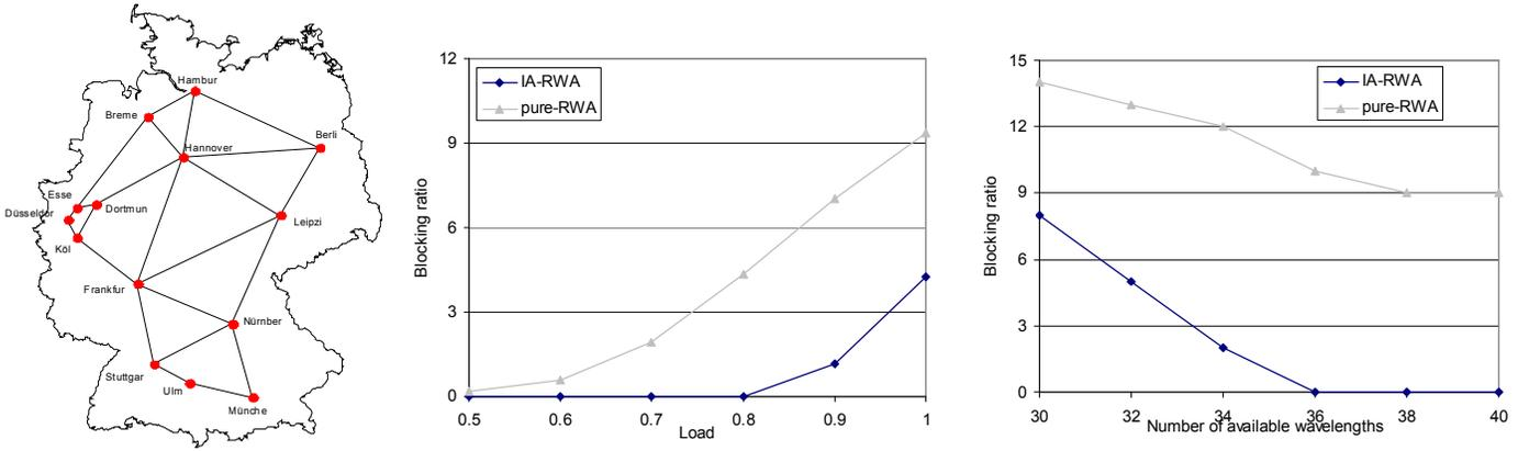
Fig. 3: (a) Generic DT network topology. 14 nodes and 23 links (we assumed 46 directed links). (b) Blocking probability vs. load assuming  $W=16$  available wavelengths. (c) Blocking probability vs. the number of available wavelengths  $W$ , for realistic traffic load.
