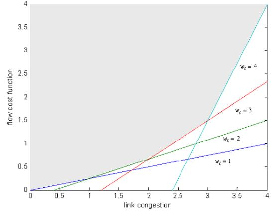
Fig. 1: The set of linear constraints that are inserted in LP formulation. We use inequality constraints to limit our search in the colored area. Since the objective that is minimized is the flow cost, we finally search for solutions only at its lower bounds, which identify the piecewise linear approximation of  $F_l$ .
