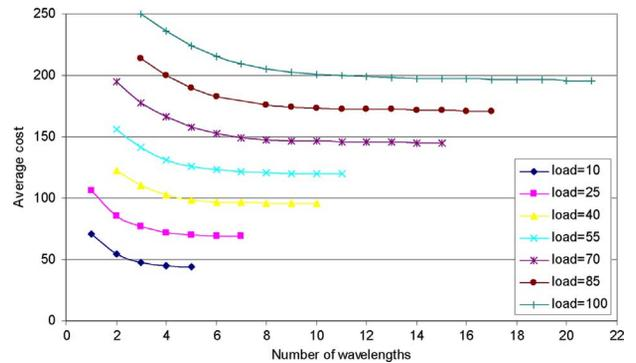
Fig. 7. Average transponders cost as a function of the number of available wavelengths for different loads found by the ILP translucent algorithm for the small-network topology.
