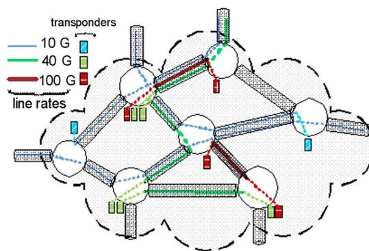
Fig. 1. Part of a network that supports mixed line rates (MLRs).
