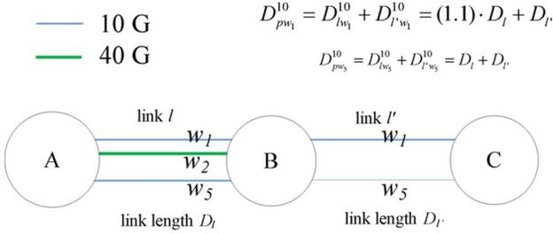
Fig. 2. Calculation of the effective length of a lightpath, taking into account the interference of other lightpaths that utilize different rates/modulation formats.
