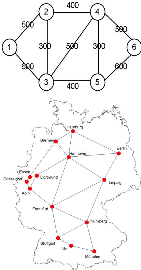
Fig. 5. (a) Six-node network topology. (b) Generic DT network topology, with 14 nodes and 23 undirected links.
