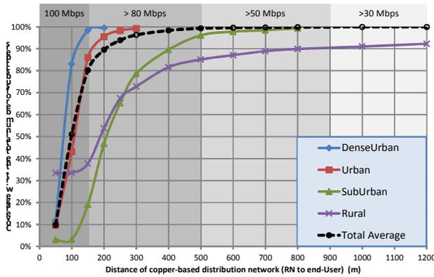
**Figure 5. Subscribers' coverage versus distribution network distance for different areas, and achievable data rates per distance for VDSL2 technology.**
