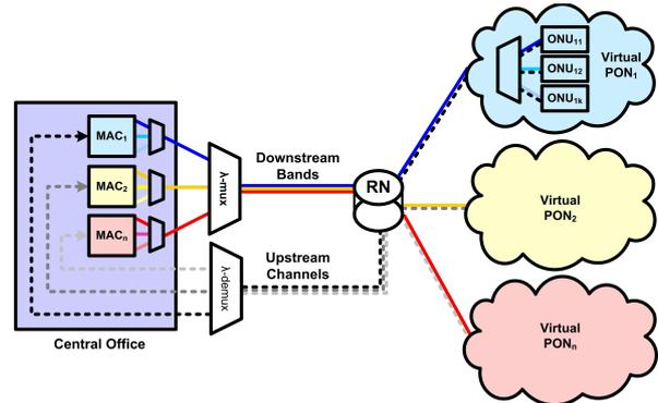
**Figure 4. Fully multiwavelength PANDA architecture.**
