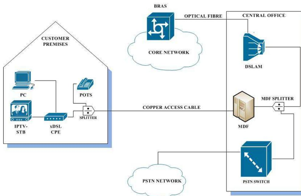
Figure 1. Broadband access via copper cables.
