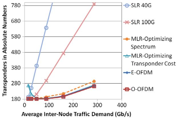
Fig. 2. (Color online) The required number of transponders is presented for different networking solutions as a function of the average inter-node traffic demand (in absolute numbers).
