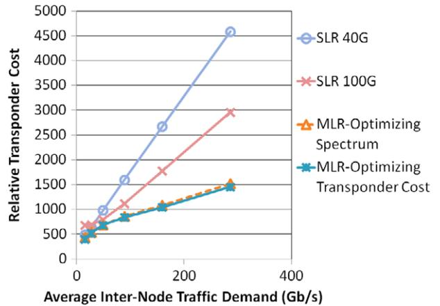
Fig. 3. (Color online) The relative transponder cost for the fixed-grid networking solutions is presented as a function of the average inter-node traffic demand. Costs are normalized to the value of one 10 Gb/s transponder.
