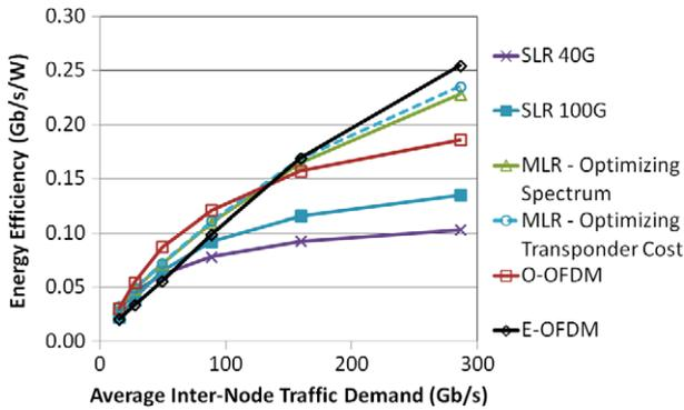
Fig. 6. (Color online) The energy efficiency achieved for different networking solutions as a function of the average inter-node traffic demand.
