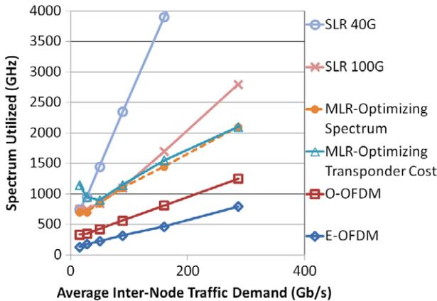
Fig. 1. (Color online) The spectrum utilization is presented for different networking solutions as a function of the average inter-node traffic demand.
