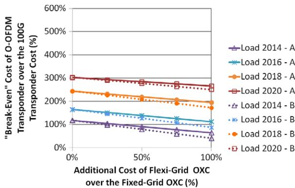
(c) The normalized cost per 50 GHz channel is set to 1 cost unit.
