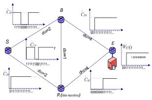
Fig. 2. A task request is forwarded to the distributed scheduler S. The task requires the transmission of a burst with duration  $b=I/C_I$  from source (which can be S or a data repository site R) and r CPUs to execute. Each link is characterized by its propagation delay (in  $\tau_I$  time units) and its binary capacity availability vector  $\hat{C}_I$ . Node E has a cluster with binary r-cluster availability vector  $\hat{W}_E(r)$ .
