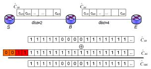
Fig. 3. Calculation of the path capacity availability vector  $\hat{C}_{SBE}$ .  $\hat{C}_{BE}$  is left shifted by  $2 \cdot d_{SB} \tau_{\Gamma}$  time units ( $d_{SB}$ =2 in this example), before the AND operation is applied.
