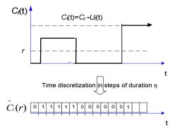
Fig. 1. The capacity availability profile  $C_l(t)$ , and the binary r-capacity availability vector  $\hat{C}_l(r)$  of a link l of capacity  $C_l$ . In a similar way we can define the cluster availability profile  $W_m(t)$  and the binary r-cluster availability vector  $\hat{W}_m(r)$ .
