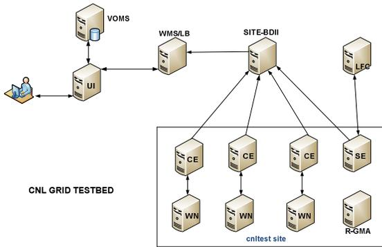
Figure 4. The gLite testbed used in our experiments.
