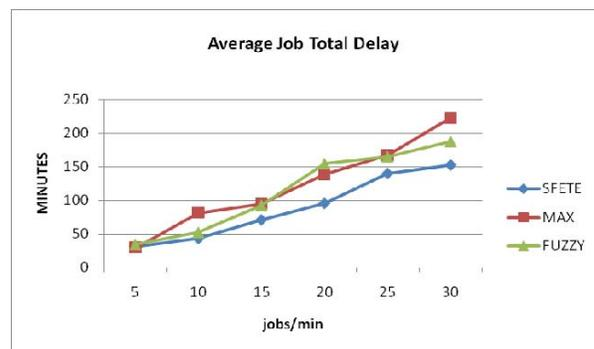
Figure 5. The average job total delay for the Max Rank, the Fuzzy Rank and the SFETE algorithms, for various job submission rates.
