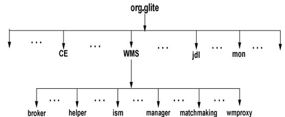
Figure 2. The structure of the gLite's directories where the WMS code is located.
