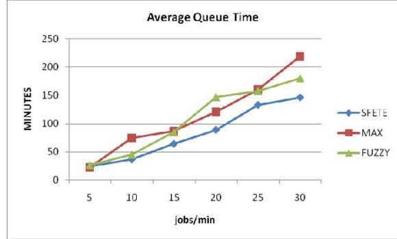
**Figure 7. The average time jobs remain at the queues of the CEs for the Max Rank, the Fuzzy Rank and the SFETE algorithms, for various job submission rates.**
