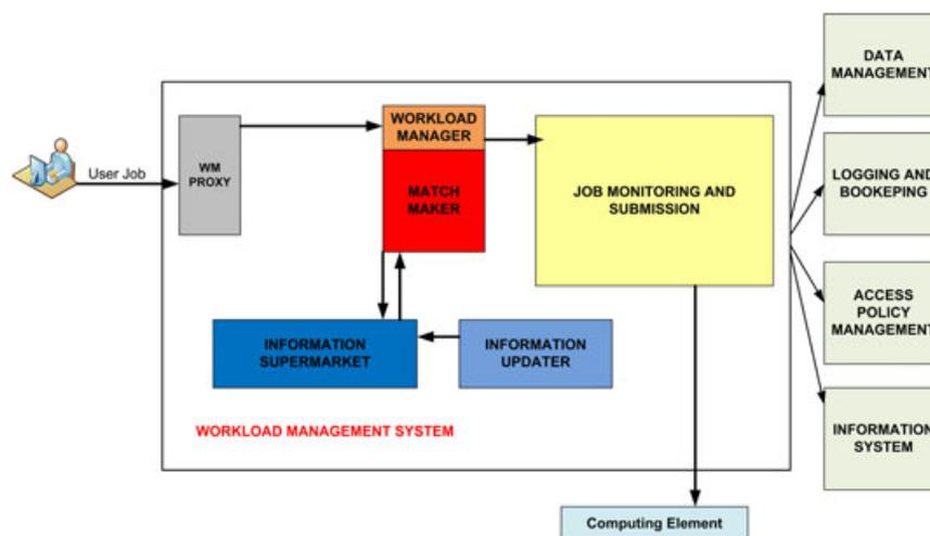
Figure 1. The gLite WMS architecture and the internal synergy of the WMS components.
