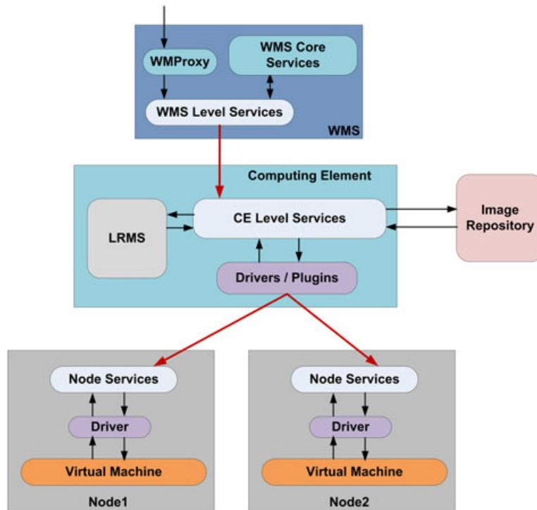
Figure 3. Virtual WN mechanism's components and their interaction.
