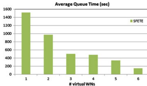
Figure 11. The average time jobs remain at the queues of the CEs using the SFETE algorithm enhanced with the virtual WN mechanism as a function of the maximum number of allowed virtual WNs per resource and for job submission rate equal to 15 jobs/s.
