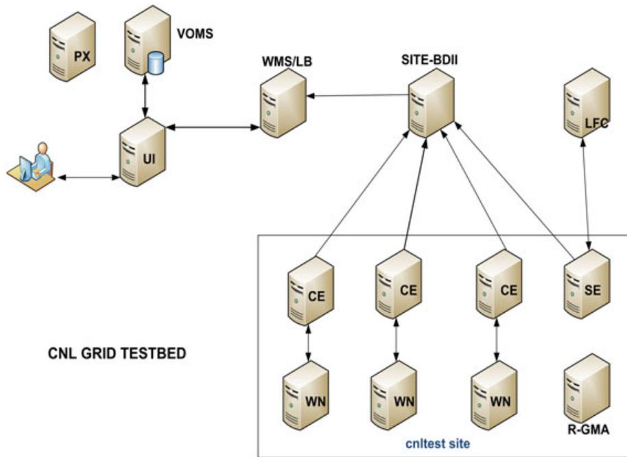
Figure 7. The gLite testbed used in our experiments.
