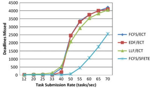
Figure 6. Deadlines missed versus the task submission rate.
