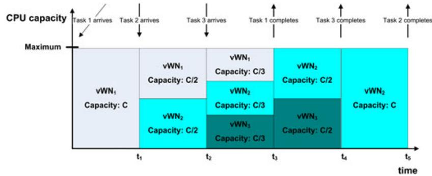
Figure 2. The virtual WNs and their computational capacities as new jobs arrive in the resource or complete their execution.
