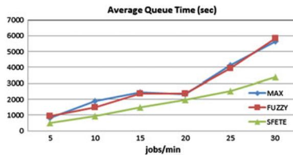
Figure 10. The average time jobs remain at the queues of the CEs for the Max Rank, the Fuzzy Rank and the SFETE algorithms as a function of the job submission rate.
