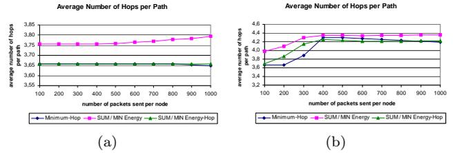
**Figure 5.** Illustrates the average number of hops of the paths followed for the *Minimum-Hop*, *SUM/MIN Energy* and *SUM/MIN Energy-Hop* algorithms. The results were obtained for the case of (a) infinite and (b) finite energy and the topology of Figure 1a
