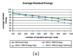
**Figure 9.** Illustrates the average residual energy for the *Minimum-Hop*, *MAX/MIN Energy* and *MAX/MIN Energy-Hop* algorithms. The results were obtained for the case of infinite energy and the topology of the simple  $7 \times 7$  grid (transmission range fixed at 50 metres).
