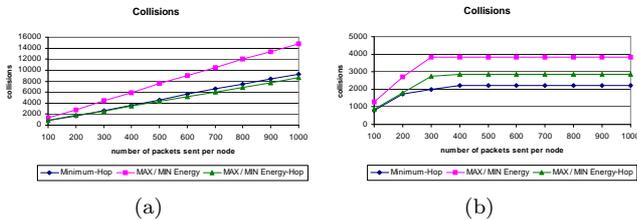
**Figure 7.** Illustrates the number of collisions for the *Minimum-Hop*, *MAX/MIN Energy* and *MAX/MIN Energy-Hop* algorithms. The results were obtained for the case of (a) infinite and (b) finite energy and the topology of Figure 1a.
