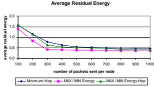
**Figure 2.** Illustrates the average residual energy at the end of the evacuation problem for the *Minimum-Hop*, *MAX/MIN Energy* and *MAX/MIN Energy-Hop* algorithms. The results were obtained for the case of finite energy and the topology of Figure 1a.
