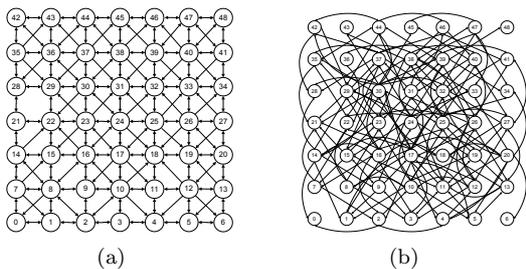
**Figure 1.** Illustrates (a) Network topology when the transmission range of the nodes varies between 50m-100m and (b) Network topology when the transmission range of the nodes varies between in the range 50m-150m (we omit the edges that have already been shown in the previous topology figure).
