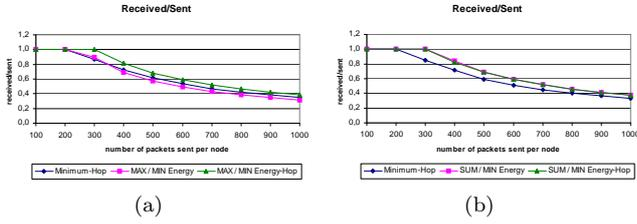
**Figure 6.** Illustrates the received received-to to-sent packets ratio for the *Minimum-Hop* and (a) *MAX/MIN Energy*, *MAX/MIN Energy-Hop* and (b) *SUM/MIN Energy* and *SUM/MIN Energy-Hop* algorithms. The results were obtained for the case of finite energy and the topology of Figure 1a.
