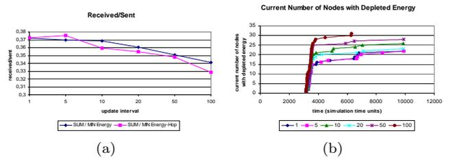
**Figure 8.** Illustrates (a) the received to sent packets ratio and (b) the current number of nodes with depleted energy for the *Minimum-Hop*, *SUM/MIN Energy* and *SUM/MIN Energy-Hop* algorithms. The results were obtained for the case of finite energy and the topology of Figure 1a.
