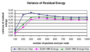
**Figure 3.** Illustrates the variance of the residual energy at the end of the evacuation problem for the *Minimum-Hop*, *SUM/MIN Energy* and *SUM/MIN Energy-Hop* algorithms. The results were obtained for the case of finite energy and the topology of Figure 1a.
